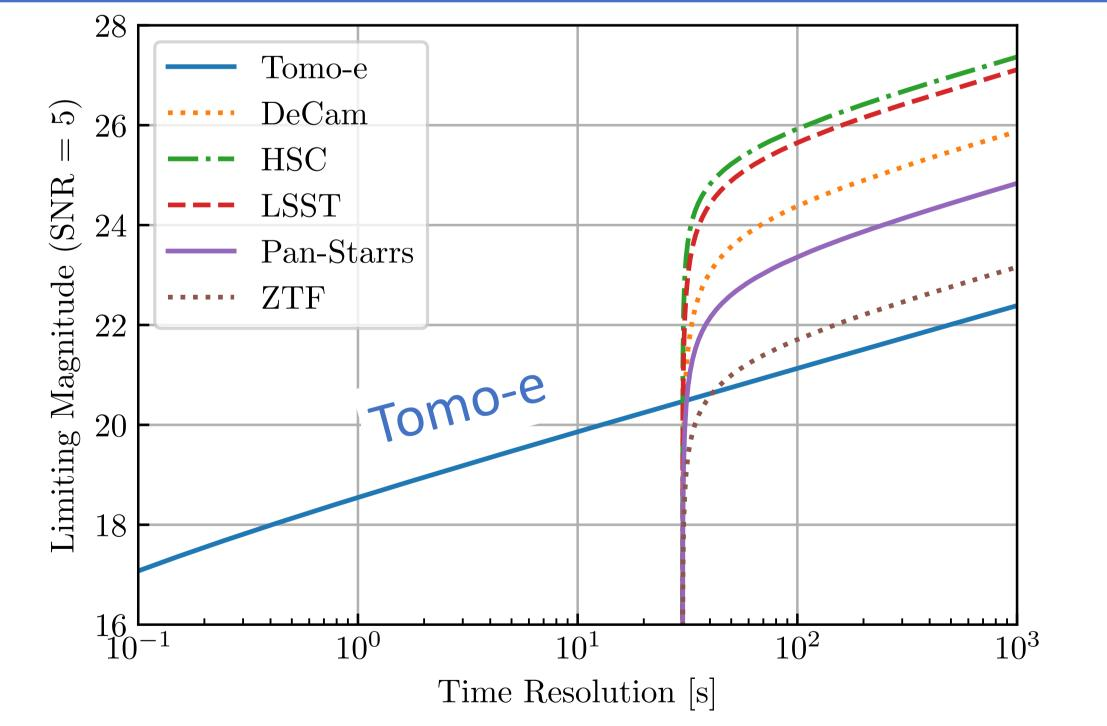
Fig. 2 Sensitivities of optical telescopes with different time resolution.
