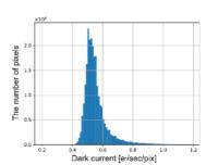
Figure 4. Distribution of the dark current at 290 K
