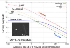
Figure 7. Limiting magnitudes to a fast moving object with Tomo-e Gozen and wide field instruments
