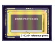
Figure 2. Canon 35MMFHDXM 35 mm CMOS sensor
