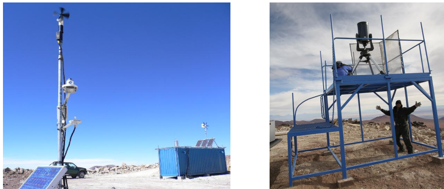
Figure 6. (Left) The meteorological weather tower and a container installed at the summit. The cloud monitor and solar panels are placed on the container. (Right) The DIMM system on the 2m tower used to measure the seeing size.
