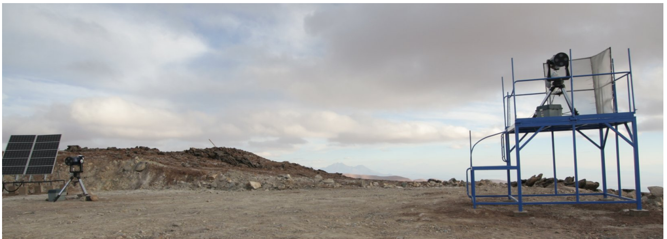
Figure 5. Two UT-DIMMs were set up at the summit of Co. Chajnantor for the simultaneous observations during the Apr. 2007 run, where one DIMM is set on the 2m tower to avoid the effect of the ground layer turbulence. The DIMM on the ground is installed at the same place as the run of Nov. 2007.
