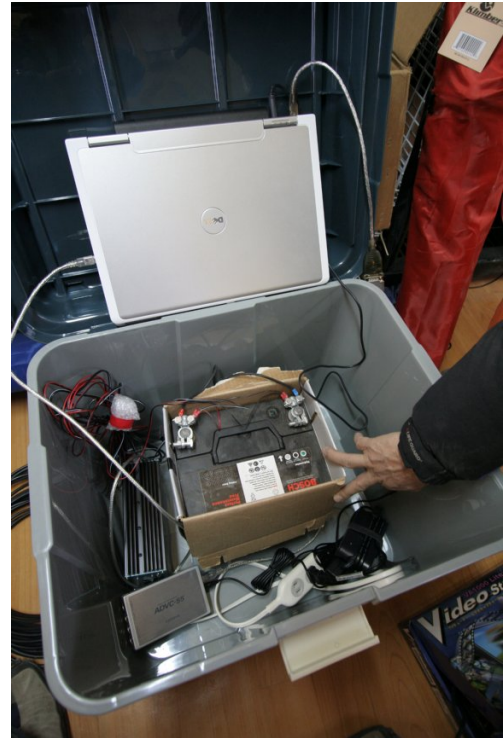
Figure 4. (Right) The data acquisition system of UT-DIMM. The car batter is placed at the middle of the box, while the DC-AC inverter is seen left to it. The DV converter is the small box lower to the inverter, and the Laptop PC is layed at the top.
