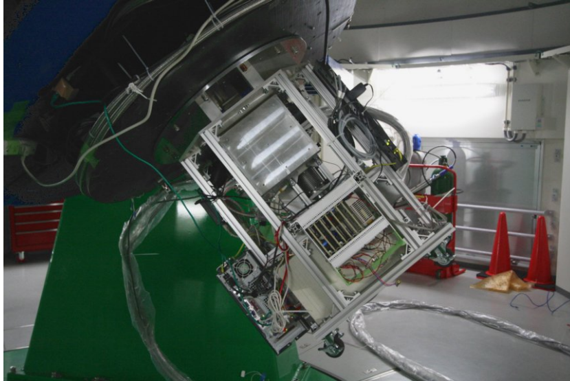
Figure 10. ANIR mounted on the Cassegrain focus of the 1.5m “Kanata” telescope at the Higashi-Hiroshima Observatory.
