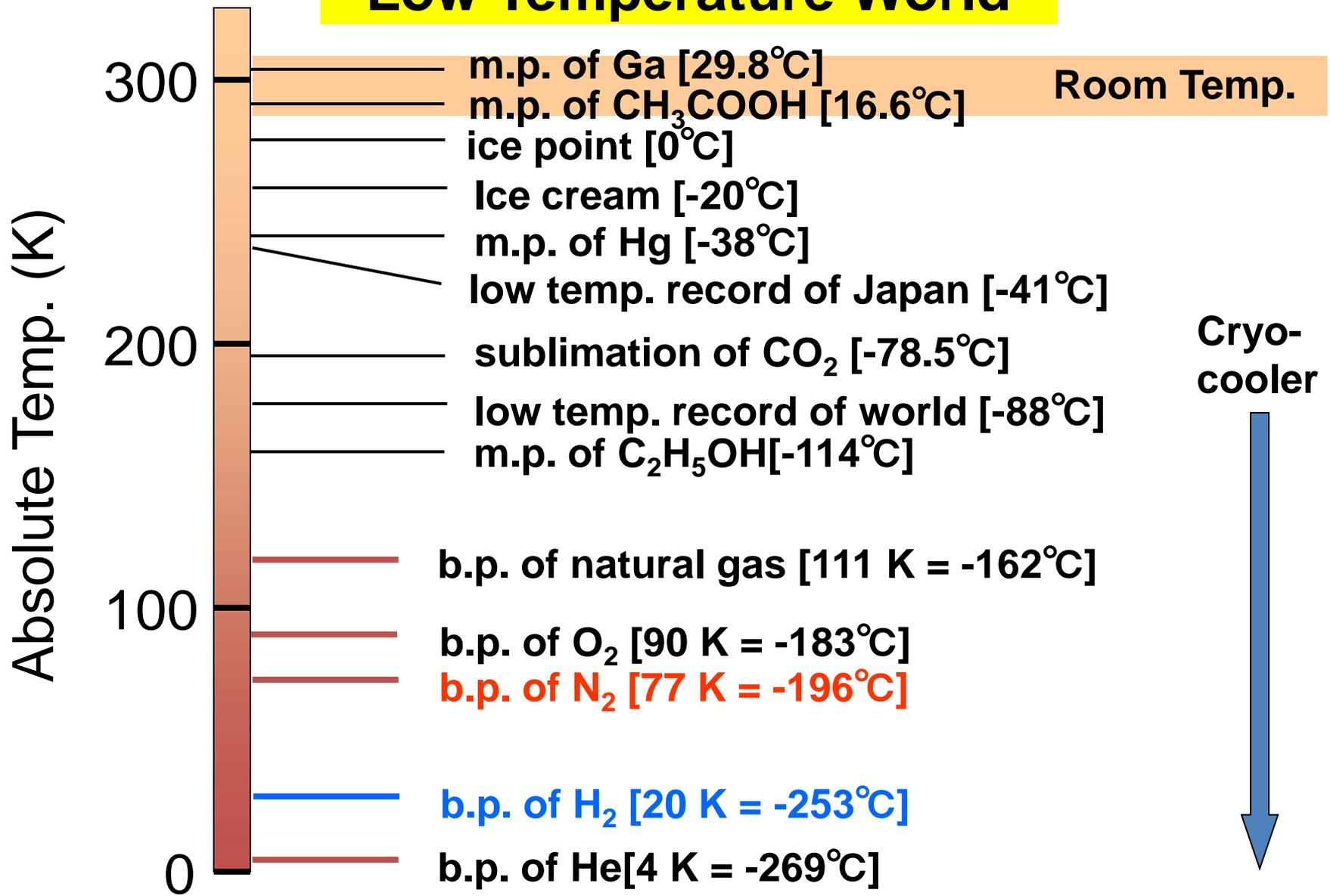
Liq. N<sub>2</sub>: 66 K(low *p*)~77.3 K(1 bar)、liq. H<sub>2</sub>: 14 K(low *p*)~20.3 K(1 bar)
