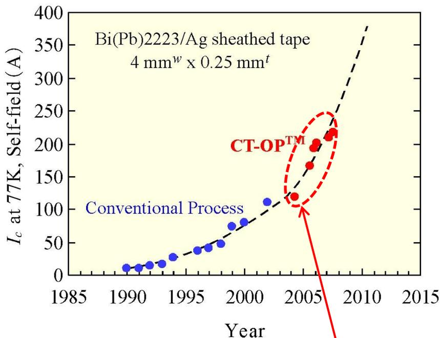
Homogeneous properties over long tapes enabled optimization of synthesis conditions
