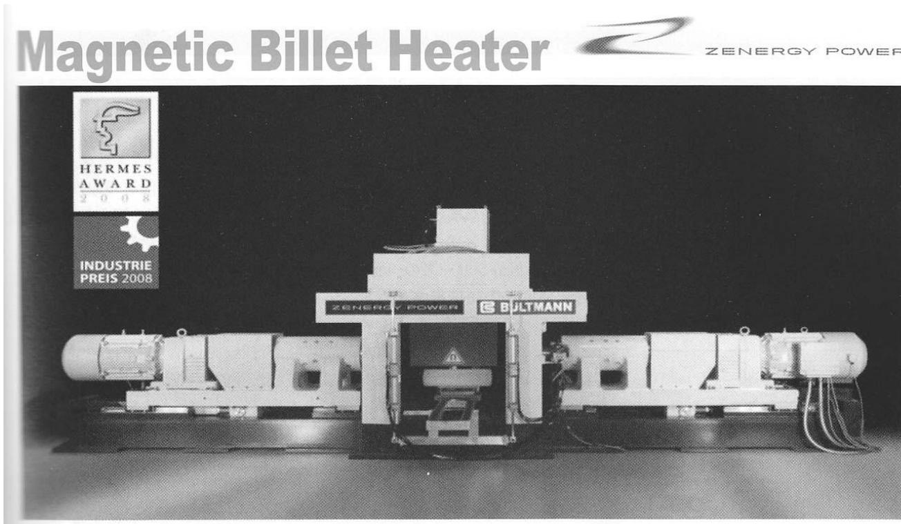
Induction heating of metal billet in Bi2223 coils → extrusion molding
