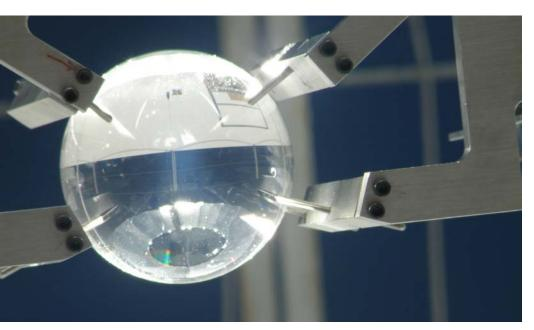
The sunlight from each dish is focused in the center of a sphere of pure fused silica - the blue glow is Rayleigh scattering
