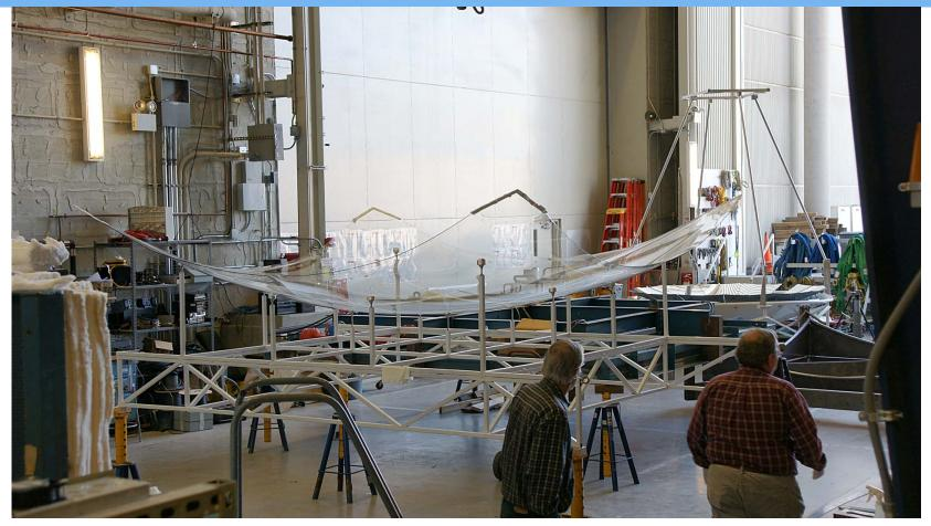
First slumped 3m x 3m reflector. Process still under development. Also need efficient means of backside coating with silver and applying protective covering. Individuals shown are Roger Angel and Materials Scientist, Blane Olbert.
