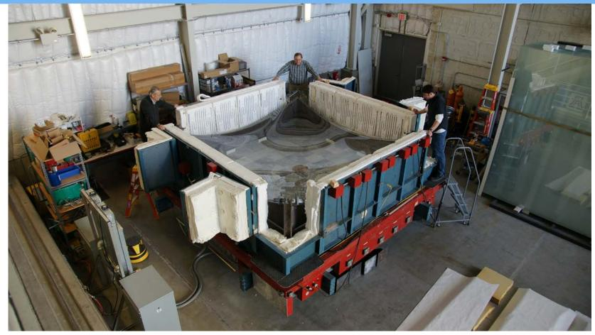
The prototype slumping furnace in the UA Mirror Lab. In production, the float glass sheets need to be slumped at same rate, 1 per 10 seconds, as they are produced. At that rate can build capacity of ~7.5 Gigawatts per year per float glass factory.
